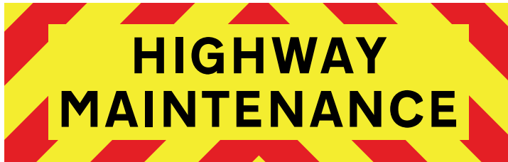
2000mm x 700mm Chevron Panel Chevron Width 150mm and positioned at 45° HIGHWAY MAINTENANCE at 100mm Xheight
