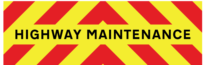
2000mm x 700mm Chevron Panel Chevron Width 150mm and positioned at 45° HIGHWAY MAINTENANCE at 100mm Xheight
